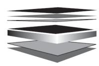
Finish Coat (Nominal 14µm) (Refer Note 4 & 5) Universal Corrosion Inhibitive Primer (Nominal 3µm) **Conversion Coating**
