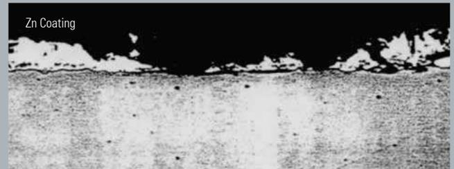
Figure A - Microscopic view of galvanized steel
