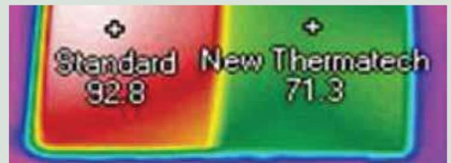
Comparison of heat radiation levels into a building interior after weathering:
