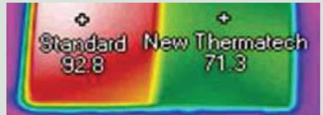
Comparison of heat radiation levels into a building interior after weathering:
