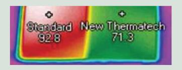
Comparison of heat radiation levels into a building interior after weathering:
