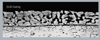
Figure B - Microscopic view of ZINCALUME® steel
