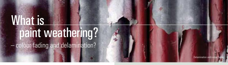
Colour fading is caused by the degradation of the key ingredients in the paint system, e.g. pigments and resins, which is due to prolonged weathering and poor formulation. Delamination is the separation of the top coat from the primer and can be caused by UV effects, poor surface preparation, poor paint formulation, or poor paint / primer specification.
