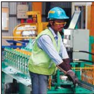
Truss components are manufactured
