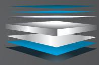
Finish Coat (Nominal 20 µm) Corrosion Inhibitive Primer (Nominal 5 µm) Conversion Coating
