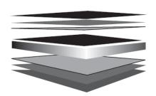
Finish Coat (Nominal 20µm) (Refer Notes 4 & 5) Universal Corrosion Inhibitive Primer (Nominal 5µm) **Conversion Coating**
