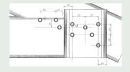
Heel Bearing Test of C75 1.0mm BMT Section with Short Stiffener and 9 off #12-14x20 Teks
