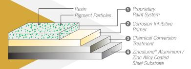
More importantly, the Proprietary Paint System has a high degree of resin stability, colour stability and UV resistance, which are the key to Colorbond® steel with Thermatech® technology's solar-reflecting properties.
