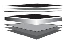
Finish Coat (Nominal 20μm) (Refer Note 4 & 5) Universal Corrosion Inhibitive Primer (Nominal 5μm) Conversion Coating
