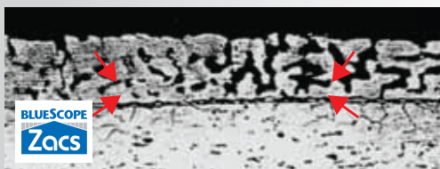
AZ90 (90g salutan lapisan aluminium-zink aloi setiap m 2 ) AZ90 (每平方公尺含90g铝锌镀层)
