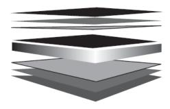
Finish Coat (Nominal 20µm) (Refer Note 4 & 5) Universal Corrosion Inhibitive Primer (Nominal 5µm) Conversion Coating
