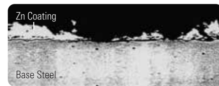
Figure A - Microscopic view of galvanized steel
