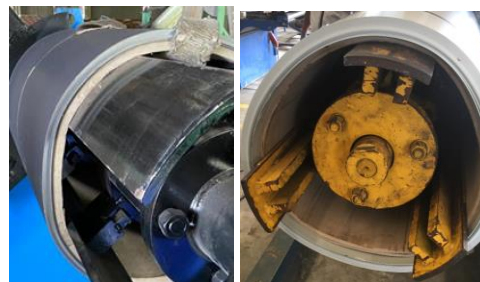
Figure 3: Over expanded mandrel caused by inconsistent torque transmission from mandrel to coil.
