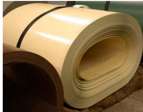
Figure 1: Coil slump (horizontal position)
