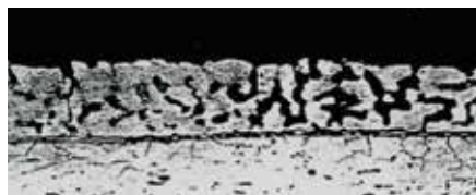
Microscopic picture view of ZINCALUME® steel after weathering
