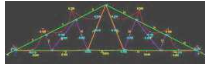
ENDUROCADD® prepares a structural analysis of the trusses following the selected loads.
