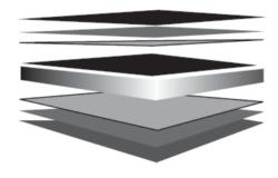
Finish Coat (Nominal 20  $\mu m)$  (Refer Note 4 & 5) Universal Corrosion Inhibitive Primer (Nominal 5  $\mu m)$  Conversion Coating
