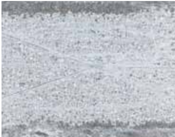
TRUECORE® steel at 500 hours
