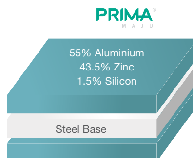
Aluminium-zinc alloy layer (AZ100 coating)
