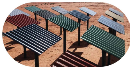
Real-World Exposure Tests 10,000 panels tested at 22 sites globally, including severe marine environments.
