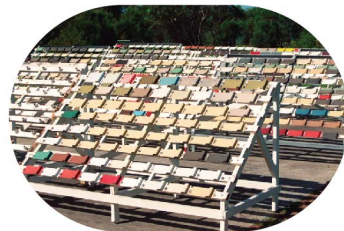
On-going exposure testing at Bellambi Point, Wollongong, Australia
