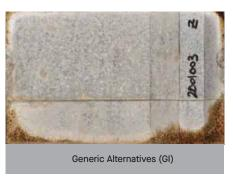
Corrosion Performance of Coated Steel After 5 Years at a Severe Marine Site (Bellambi Point, Australia).
