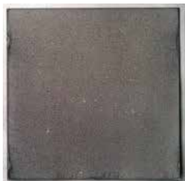
Zincalume® steel (No Sign of Rust)
