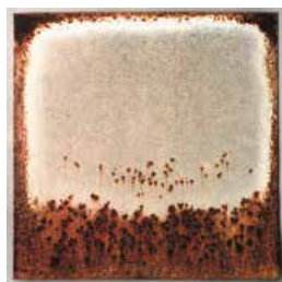
Galvanised steel Z275 (Heavy sign of Rust)
