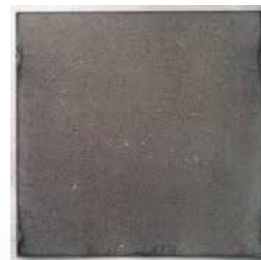
Zinalume® steel (No Sign of Rust)
