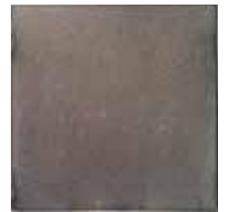
ZINCALUME® steel (No Sign of Rust)
