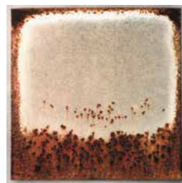
Galvanised steel Z275 (Heavy sign of Rust)
