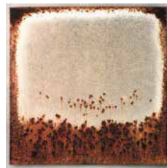
Galvanised steel Z275 (Heavy sign of Rust)
