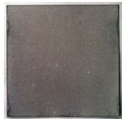
ZINCALUME® steel (No Sign of Rust)
