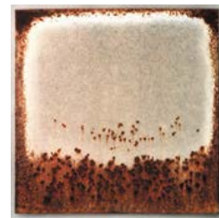
Galvanised steel Z275 (Heavy sign of Rust)
