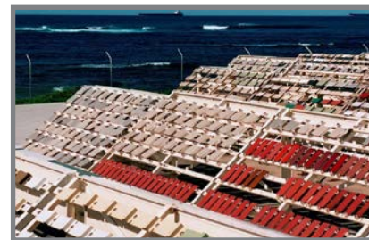
Mẫu phơi tại Bellambi Point, Wollongong, Úc Exposed panels at Bellambi Point, Wollongong, Australia
